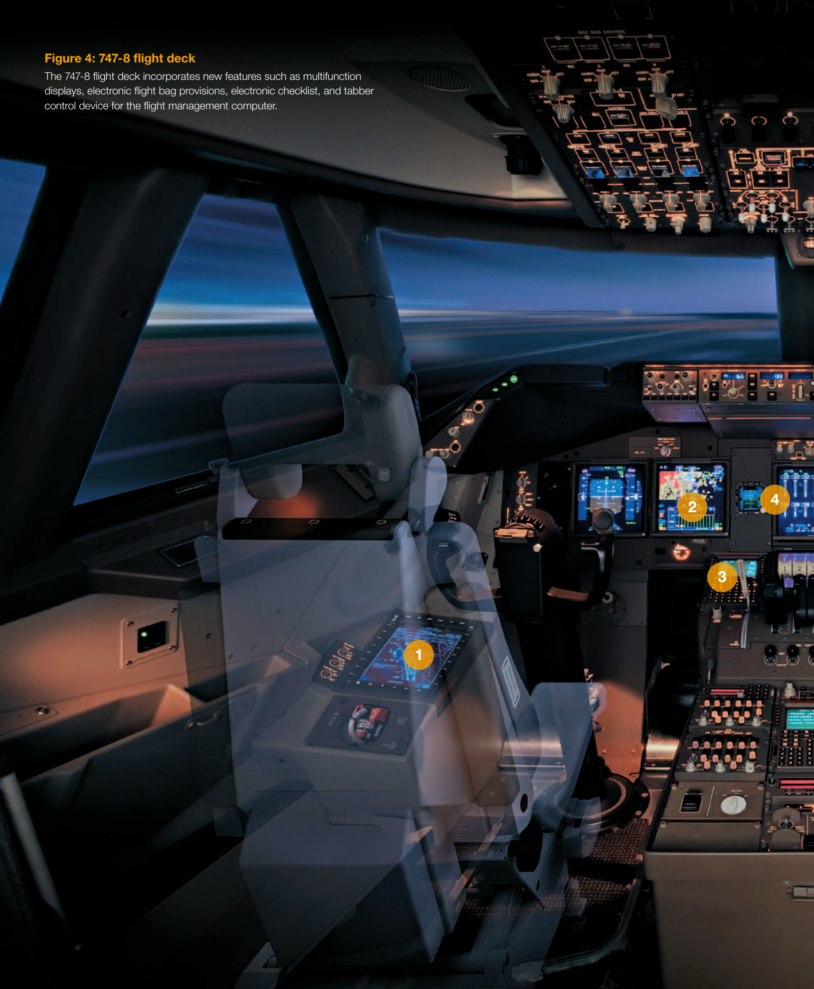
1. Electronic Flight Bag 2. Vertical Situation Display 3. Flight Management Computer 4. Electronic Checklist 5. Airport Moving Map
