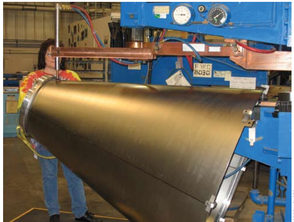
Sherry Durham, Advanced Metal Structures assembly cell technician at Boeing Auburn, and a spot welding robot position and weld parts to build a tail cone muffler for the 787 Dreamliner.
