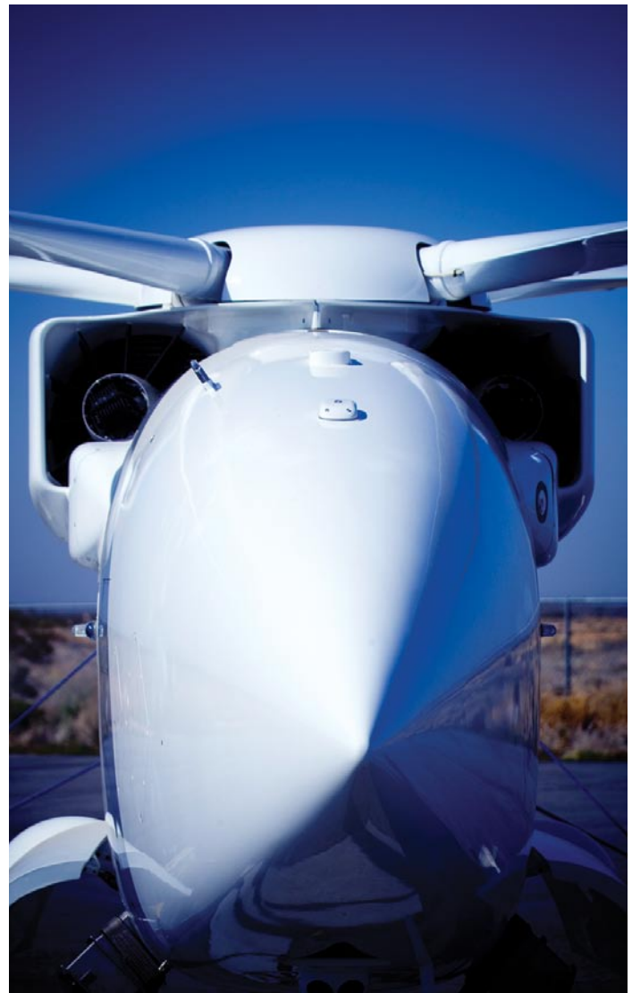
The A160 Hummingbird is being tested at Victorville, Calif. This unmanned aerial vehicle has the capability of flying at higher altitudes and traveling longer distances than current helicopters.
