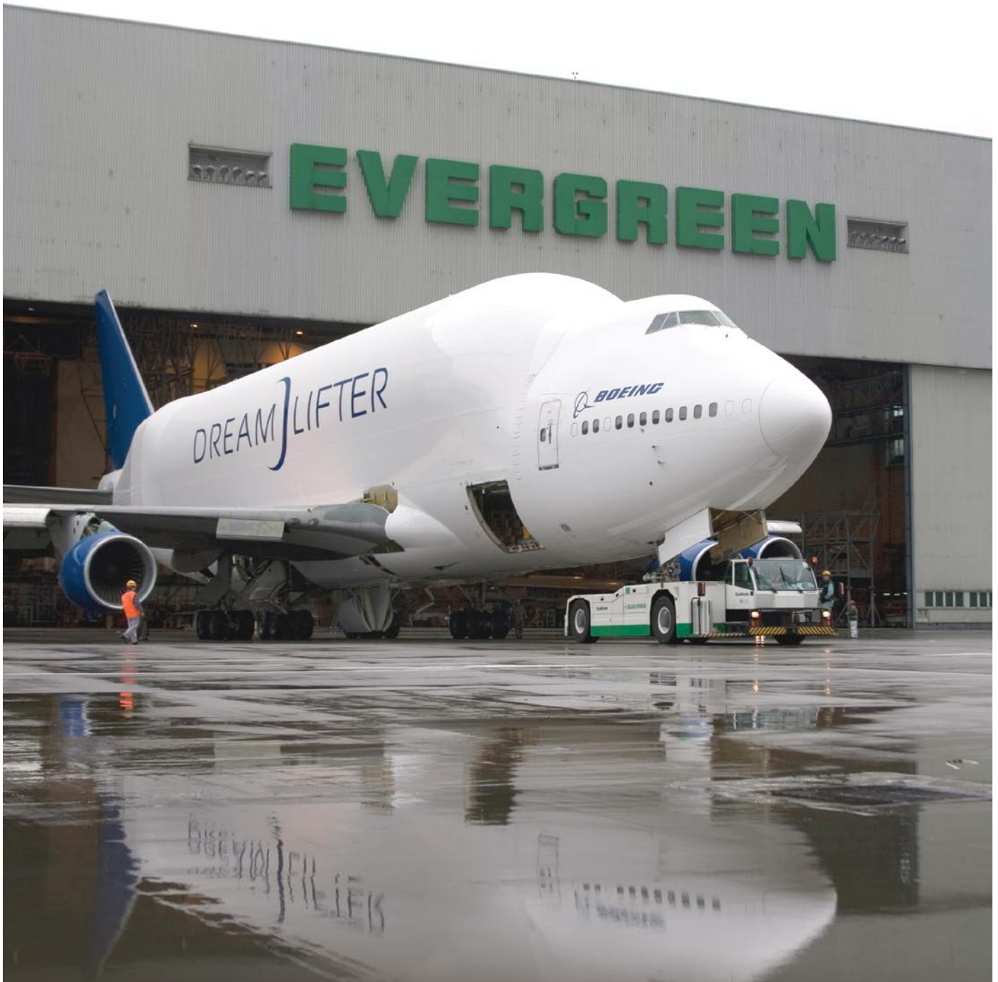
The second Dreamlifter, a specially modified 747-400 designed to carry large components of the new 787 Dreamliner airplane, rolled out of the hangar Jan. 7 in Taipei, Taiwan. The Dreamlifter plays a major role in the production of the Dreamliner by ferrying large parts of 787s from program partners around the world to the 787's final assembly site in Everett, Wash. Evergreen Aviation Technologies Corporation will modify a total of three Dreamlifters at its facility in Taiwan. Last month, the Dreamlifter successfully delivered major assemblies from Nagoya, Japan, to Charleston, S.C.
