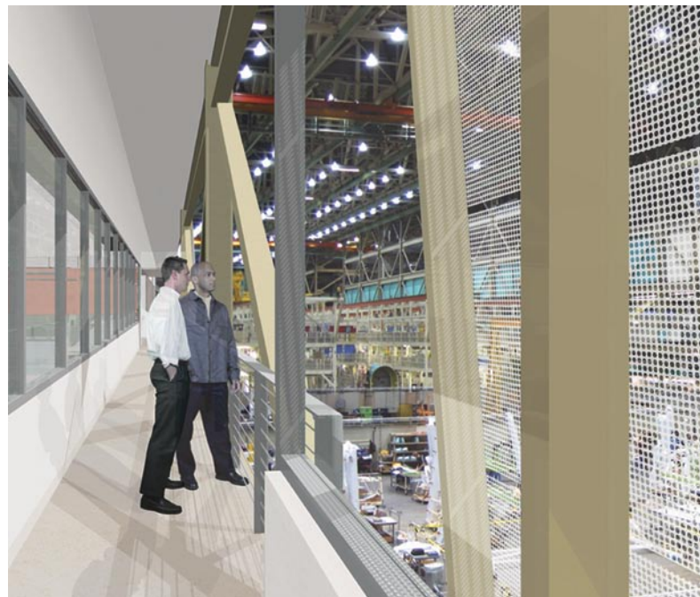
Top: This rendering depicts collaboration zones, which are areas that connect the office towers and the factory floor. They’ll offer support cells, crew break areas and other activities. The zones are intended to facilitate collaboration between factory workers and employees who design and support the products they build.
