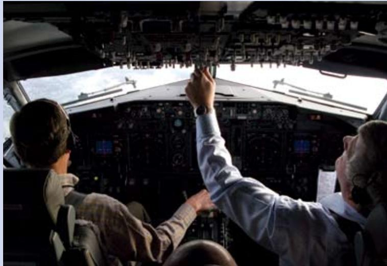
Once in flight, the pilots conduct a series of flight-test maneuvers. The crew on board—two pilots, a flight analyst and a systems operator—check systems at high and medium altitudes. They check backup and critical safety elements, including cabin pressurization and the deployment of oxygen masks, as well as avionics, navigation and communication systems, functionality of in-flight entertainment and more. They also shut down and “relight” the engines during this phase.
