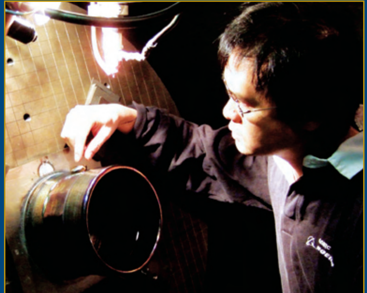
At the University of Sheffield's Advanced Manufacturing Research Centre, W.S. Tham inspects a part recently completed on the Shape Metal Deposition Cell at the facility. The cell uses titanium wire to literally grow parts up from CAD models. Boeing is the lead member and co-founder of this site, which has helped develop, validate and transition new manufacturing technologies. AMRC PHOTO
