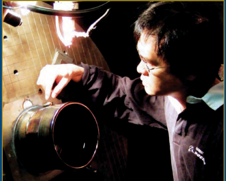
At the University of Sheffield's Advanced Manufacturing Research Centre, W.S. Tham inspects a part recently completed on the Shape Metal Deposition Cell at the facility. The cell uses titanium wire to literally grow parts up from CAD models. Boeing is the lead member and co-founder of this site, which has helped develop, validate and transition new manufacturing technologies. AMRC PHOTO
