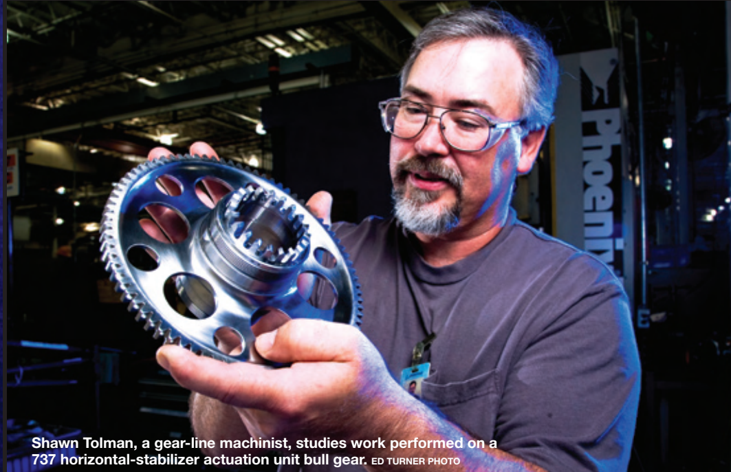
A finished bull gear for a 737 horizontal stabilizer actuation unit. ED TURNER PHOTO
