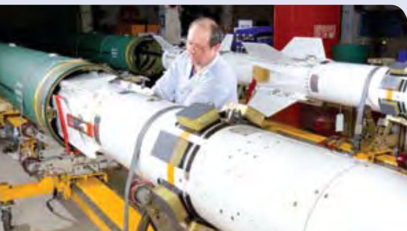
Weapons Programs employee Russell Evans prepares a Harpoon missile for installation in a submarine launch capsule. Boeing recently was awarded a system design and development contract for the Harpoon Block III missile.
