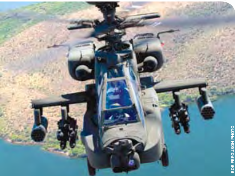
The AH-64D Apache Longbow is a multirole, heavy-attack combat helicopter that can transmit real-time digitized information to air and ground forces.
