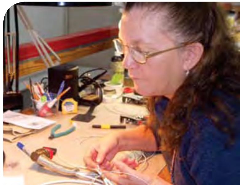
Retrofit & repair technical specialist Linda Nelson assembles an aircraft wiring harness. She's with a Boeing team in Fort Walton Beach, Fla., that provides repair and logistics services for U.S. Air Force Special Operations Forces aircraft.
