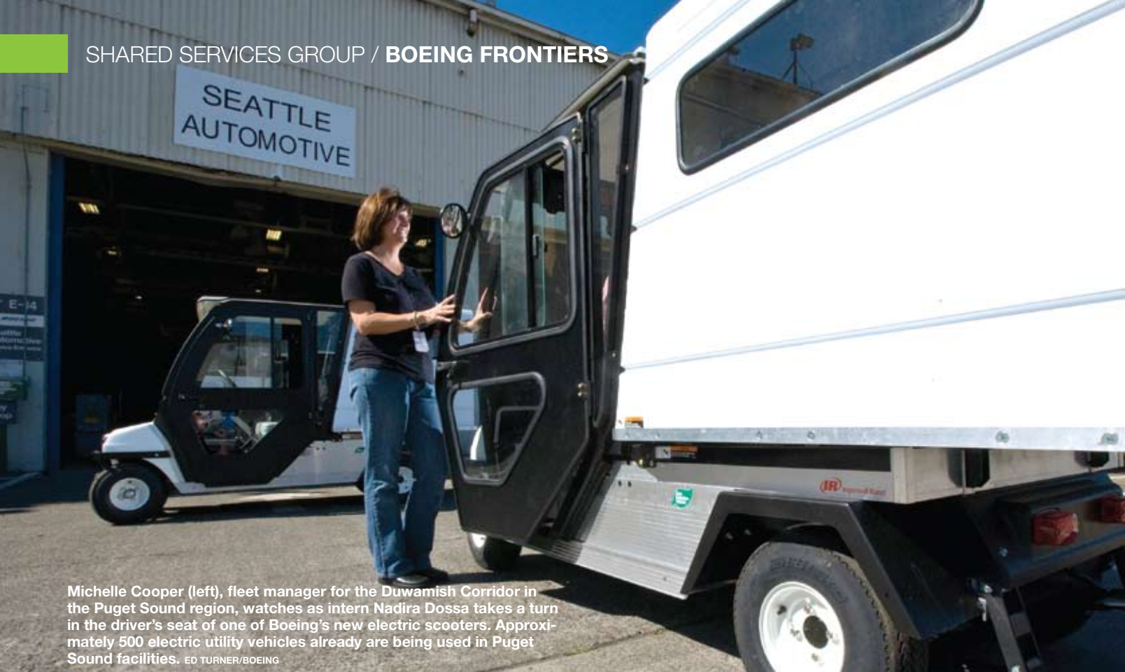
Electric utility vehicles used at Boeing plants can be recharged by pulling an electric cord from the cab and plugging it in to a standard electric outlet. ED TURNER/BOEING
