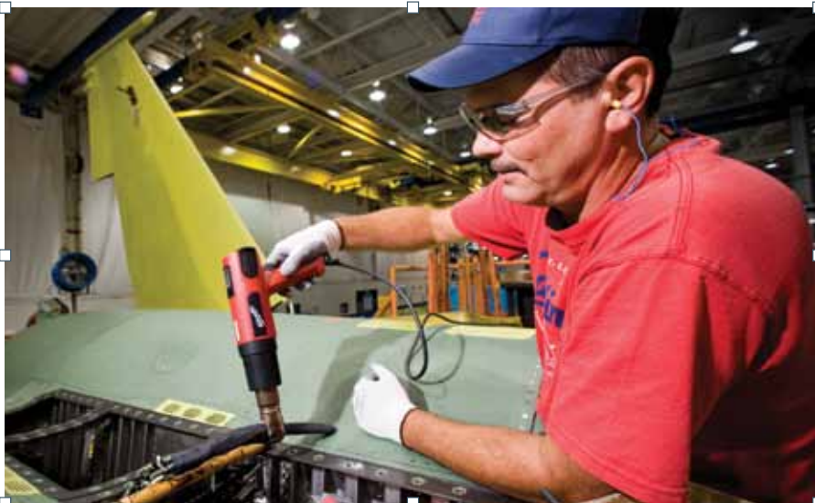
PHOTO: Electrician Barry Betz heat shrinks protective wrap over an electrical splice in an F-15 aft fuselage. PETER GEORGE/BOEING
