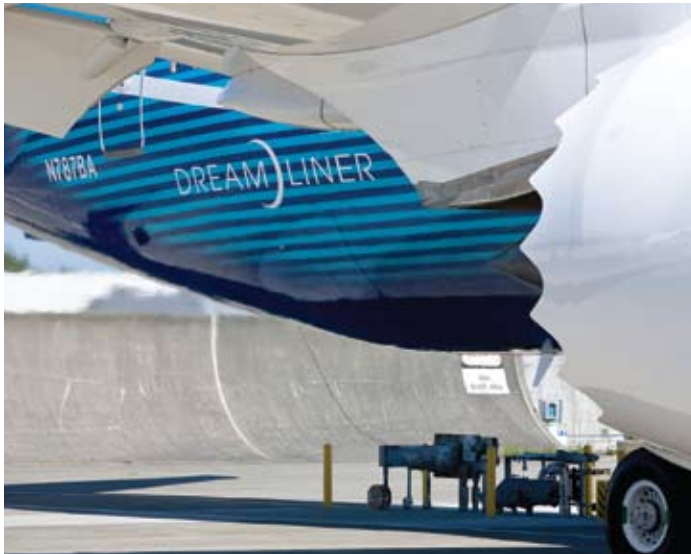
PHOTO: Specially shaped nacelle trailing edges on the 787 Dreamliner reduce engine noise to communities by controlling the way air mixes after passing through and around the engine.
