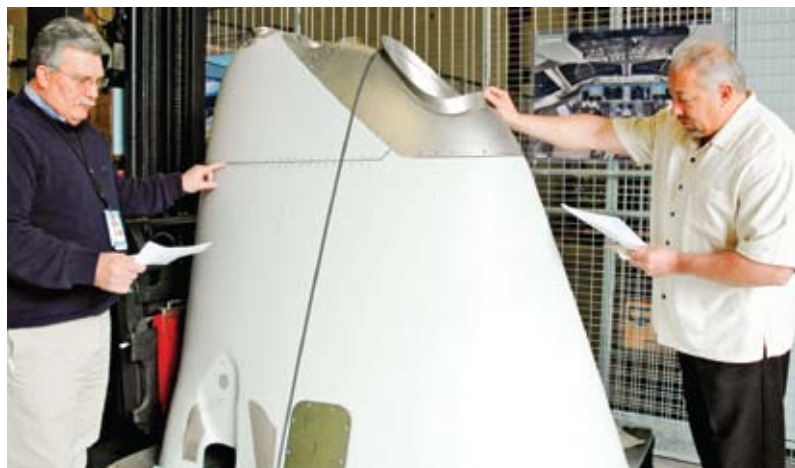
PHOTO: Boeing Enterprise Asset Resale Manager Joe Ferreri (left) and Phil Arroyo, Volvo Aero Services sales director, check the certification of a 737-700 tailcone, an excess asset created during modification of a new 737 into a Wedgetail Airborne Early Warning and Control platform. DOUG CANTWELL/BOEING
