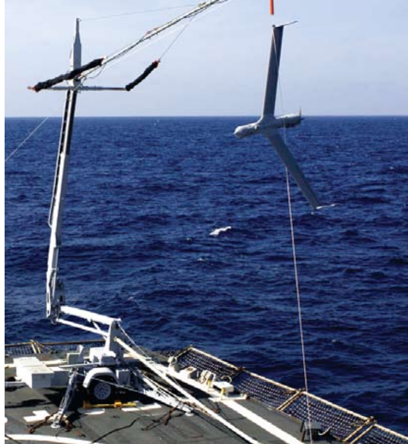
PHOTO: Nearly invisible and inaudible at its usual operating altitude of 1,500 feet (457 meters), the Boeing-Insitu ScanEagle unmanned aircraft system, shown here following a recovery aboard the destroyer USS Oscar Austin , operates from several different types of U.S. Navy vessels. A ScanEagle operated from the Oscar Austin's sister ship, USS Bainbridge , provided critical intelligence, surveillance and reconnaissance support during the tracking of Somali pirates and subsequent rescue of U.S. freighter captain Richard Phillips in April. U.S. NAVY
