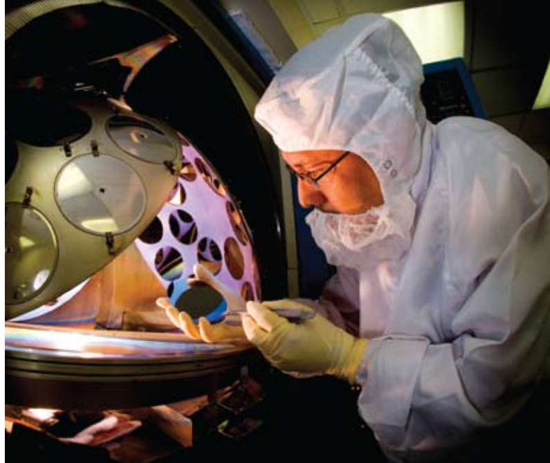
PHOTO: German Rivera, wafer processing technician at Spectrolab in Sylmar, Calif., inspects a semiconductor wafer that will yield numerous solar cells used to generate power for telecommunications satellites and spacecraft such as the Spirit and Opportunity rovers currently exploring Mars. BOB FERGUSON/BOEING
