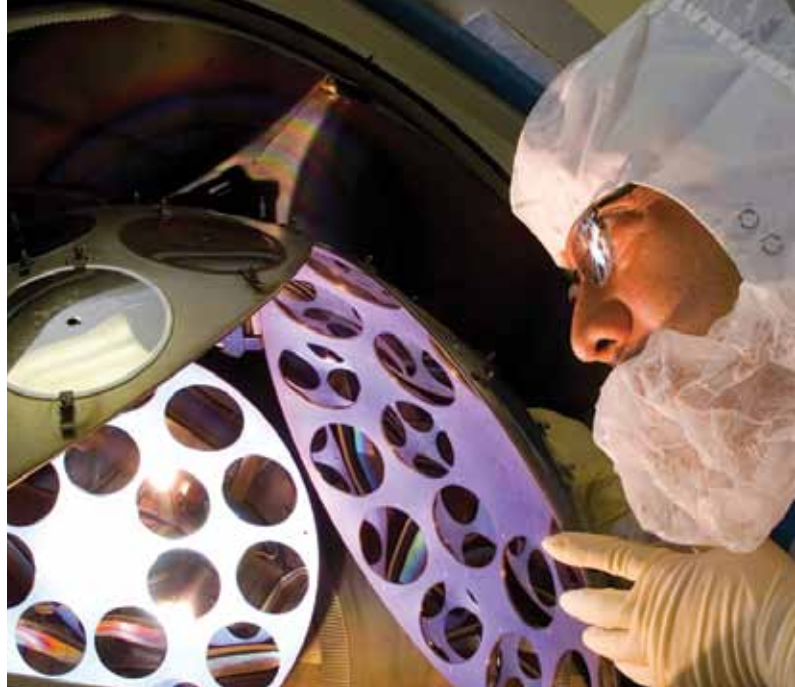
PHOTO: Wafer-processing technician German Rivera inspects a semiconductor wafer that will yield numerous solar cells used to generate power for telecommunications satellites and spacecraft such as the Spirit and Opportunity rovers currently exploring Mars. BOB FERGUSON/BOEING
