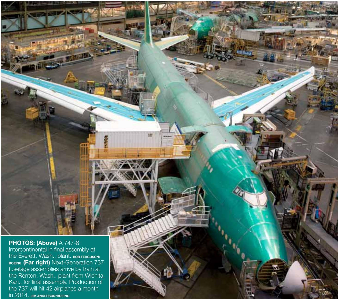
**PHOTOS: (Above)** A 747-8 Intercontinental in final assembly at the Everett, Wash., plant. **BOB FERGUSON/BOEING** **(Far right)** Next-Generation 737 fuselage assemblies arrive by train at the Renton, Wash., plant from Wichita, Kan., for final assembly. Production of the 737 will hit 42 airplanes a month in 2014. **JIM ANDERSON/BOEING**
