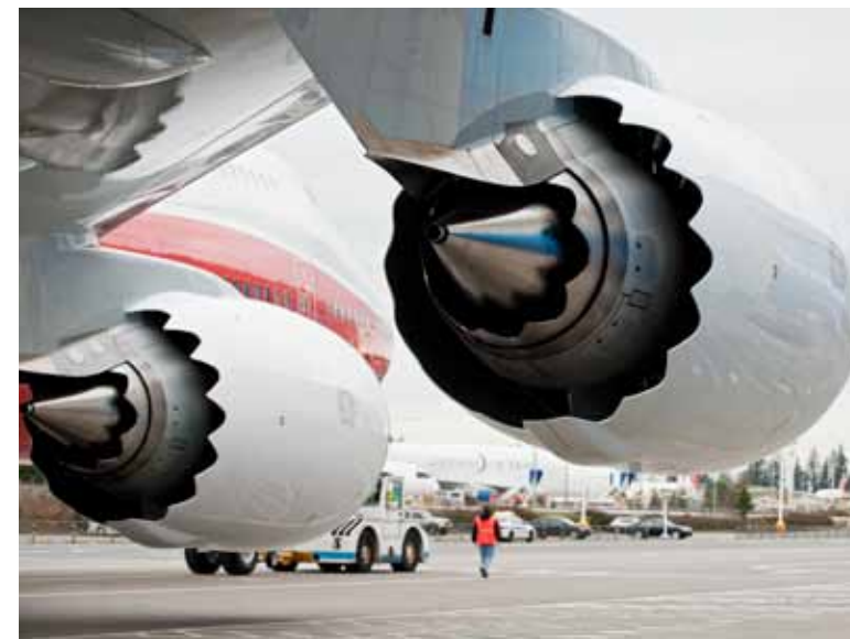
PHOTOS: (Above, from left) New fuel-efficient and quieter GENx engines boost performance of the 747-8 Intercontinental on long-haul international routes. GAIL HANUSA/BOEING The Boeing Commercial Airplanes Operations Center answers urgent service requests around-the-clock from airlines operating more than 12,000 Boeing airplanes globally. MARIAN LOCKHART/BOEING
