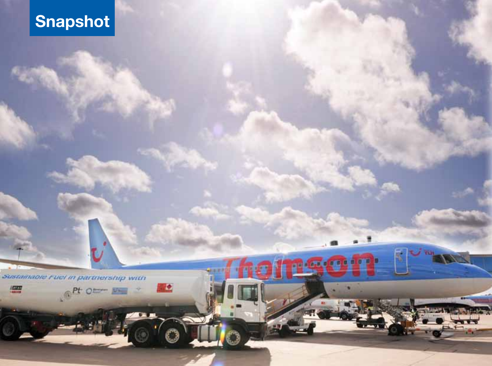
FREQUENT FRYER: A Boeing 757 operated by British charter airline Thomson Airways used a 50-50 blend of traditional jet fuel and biofuel, made from used cooking oil, to power one of its engines last month on a four-hour flight from Birmingham, United Kingdom, to Lanzarote, Spain. It carried 232 passengers and was the first revenue biofuel flight in the U.K. PHOTO: THOMSON AIRWAYS
