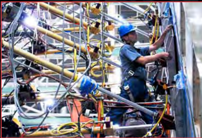
PHOTOS: (Top) As part of the F-15C full-scale fatigue test in St. Louis, the aircraft's wing is covered with tension pads bonded to the surface. BOB FERGUSON/BOEING (Insets, from left) In Everett, Wash., Dale Best prepares for the 747-8 Freighter rudder proof test, which simulates loads on the rudder surfaces; a Boeing Test & Evaluation team in Everett oversees the 747-8 Intercontinental rudder proof test. JEREMIAH SCOTT/BOEING
