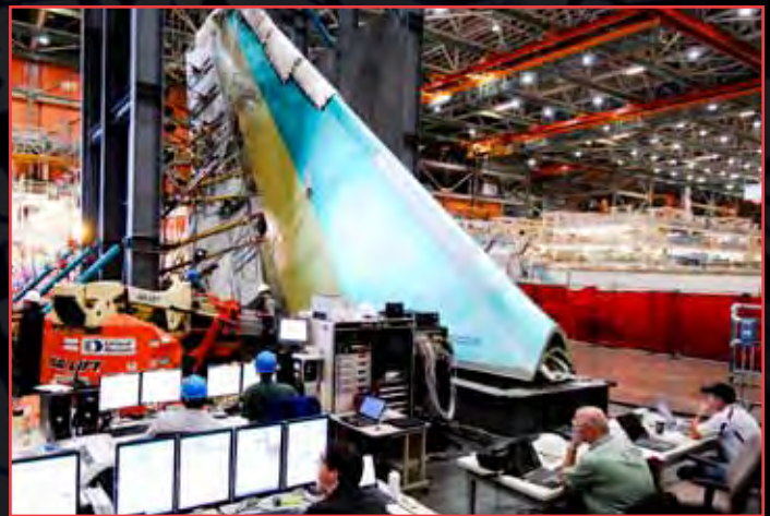
PHOTOS: (Top) As part of the F-15C full-scale fatigue test in St. Louis, the aircraft's wing is covered with tension pads bonded to the surface. BOB FERGUSON/BOEING (Insets, from left) In Everett, Wash., Dale Best prepares for the 747-8 Freighter rudder proof test, which simulates loads on the rudder surfaces; a Boeing Test & Evaluation team in Everett oversees the 747-8 Intercontinental rudder proof test. JEREMIAH SCOTT/BOEING
