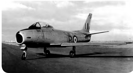
PHOTO: A Commonwealth Aircraft Corp. Sabre, built under license from North American Aviation and powered by a Rolls-Royce Avon engine. BOEING ARCHIVES
