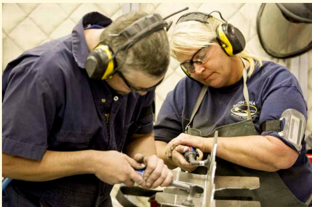
PHOTOS: (Top and middle) Tyler Blanton, Fabrication specialist, prepares a 787 side-of-body chord for installation; a 787 side-of-body chord progresses through the cutting process. BOB FERGUSON/BOEING (Above) Fabrication specialists Carl Cleveland, left, and Robin Lock hand-finish a 787 side-of-body chord to final specifications. ASSOCIATED PRESS (Far right) Matt Roddewig, Fabrication specialist, removes a 787 titanium edge frame from a computer numerical control milling machine. BOB FERGUSON/BOEING
