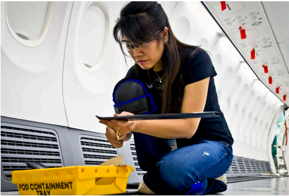
PHOTOS: Completed 737 wings are ready to be joined to the body of the airplane; Brenda Thepvangsa, 737 interiors mechanic, installs the seat cable raceway, which houses and protects entertainment system cables that run along the floor and are connected to the seats; Barry Clegg, left, of Pembroke Leasing and Leona Lyon, 737 Customer Quality Support, inspect flydubai's latest 737-800; 737 painter Jake McClain applies finishing touches to the paint scheme of flydubai's 737-800; Warren Lew, 737 interiors installation mechanic, adds Boeing Sky Interior sidewalls to a flydubai 737-800.
