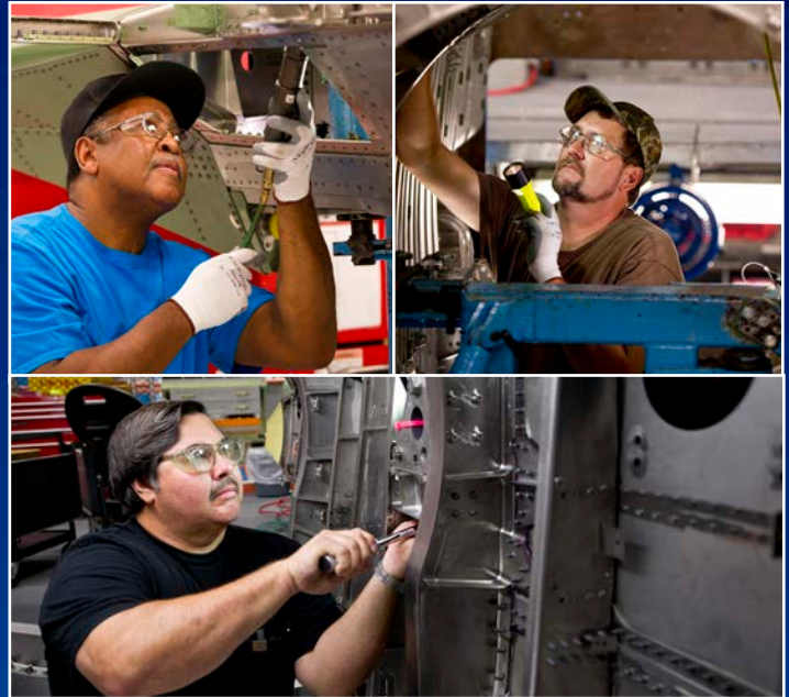
PHOTO: (Below) The F-15 Silent Eagle's stealth technology makes it less visible to an enemy's radar. BOEING (Insets) Theotric Jackson (clockwise from top left), Bob Southerland and George Louis are sheet metal assembler riveters on the F-15 line in St. Louis.
