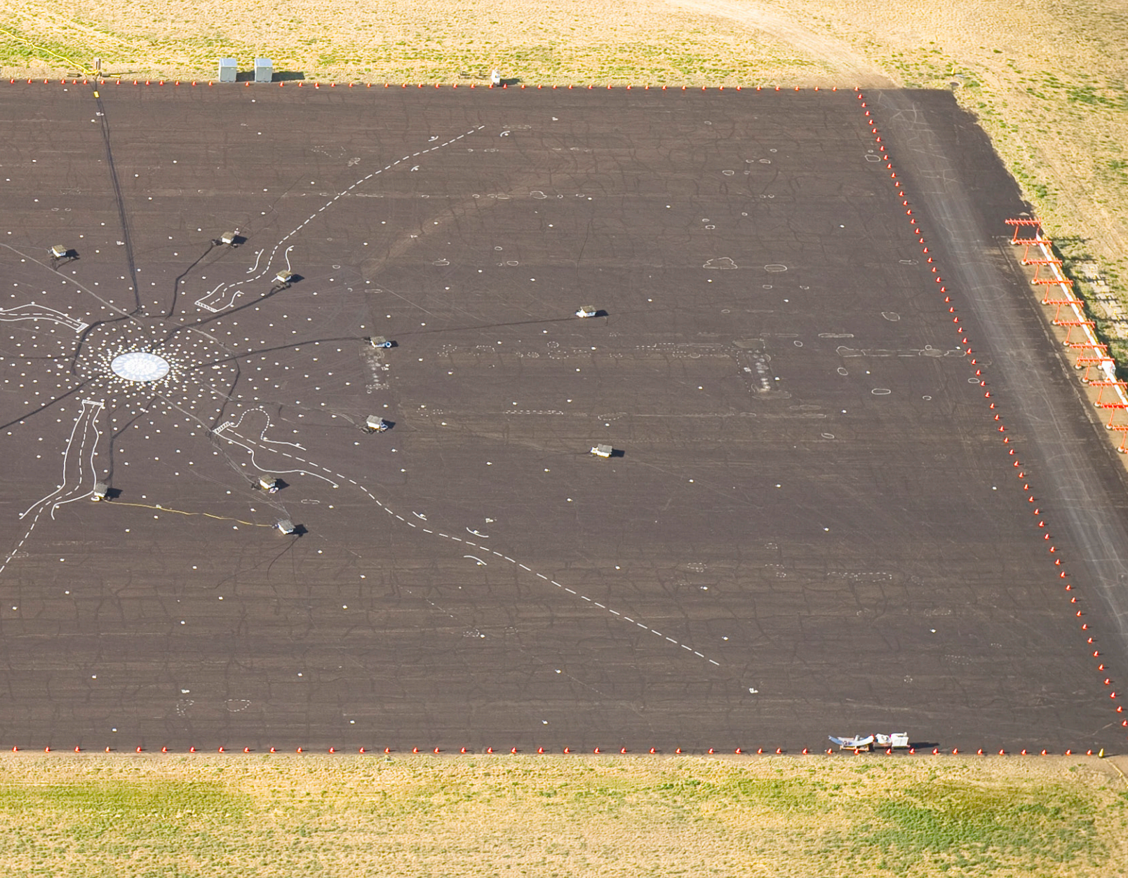
PHOTOS (Below): An aerial view of the acoustical array of microphones, used to pinpoint aircraft noise, at the end of the main runway at the Glasgow site. (Insets, clockwise from top left) The ecoDemonstrator team in Glasgow included: Steve Rapp; Tim Rahmes holding an iPad; Noel DePeralta; Dave Russell installing test sensors, Chief Pilot Mike Carriker on the flight deck; Kristin Crawford; and Kevin Johnson.
