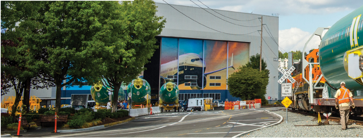
Photos: (Top) Employees stage the first 737 MAX 8 fuselage to switch tracks near the Renton, Wash., factory, where the airplane will be assembled. (Bottom, from left) Overhead crane operators lift the fuselage over to the three-story fuselage systems installation tool; the fuselage is loaded into the fuselage systems installation tool.
