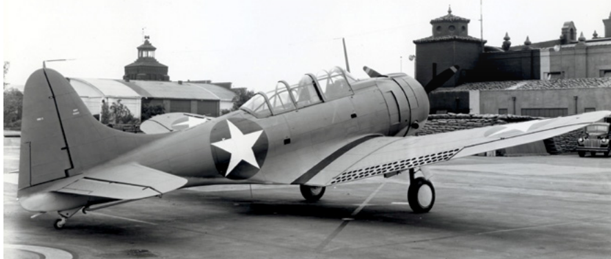
Photos: (Far left) These early production SBD Dauntless aircraft wear an overall light gray finish, which was standard until August 1941, when a U.S. Navy directive called for the upper surfaces to be painted blue-gray. (Left) The perforated dive flaps of the Dauntless can be seen on a factory-fresh SBD-3 parked on the ramp of the Douglas plant in El Segundo, Calif. BOEING ARCHIVES
