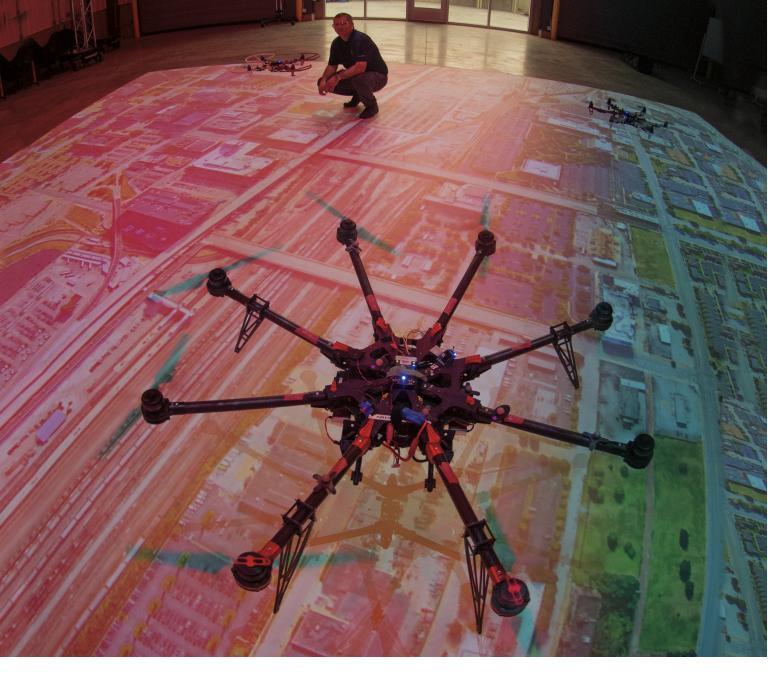
commercial building or urban area in order to use multiple unmanned aircraft systems as a problem-solver, said Tom Rice, technology lead for the Collaborative Autonomous Systems Laboratory. The lab's motion capture system covers 80,000 cubic feet (7,400 cubic meters). Protective netting separates the flight area from operators and observers.
