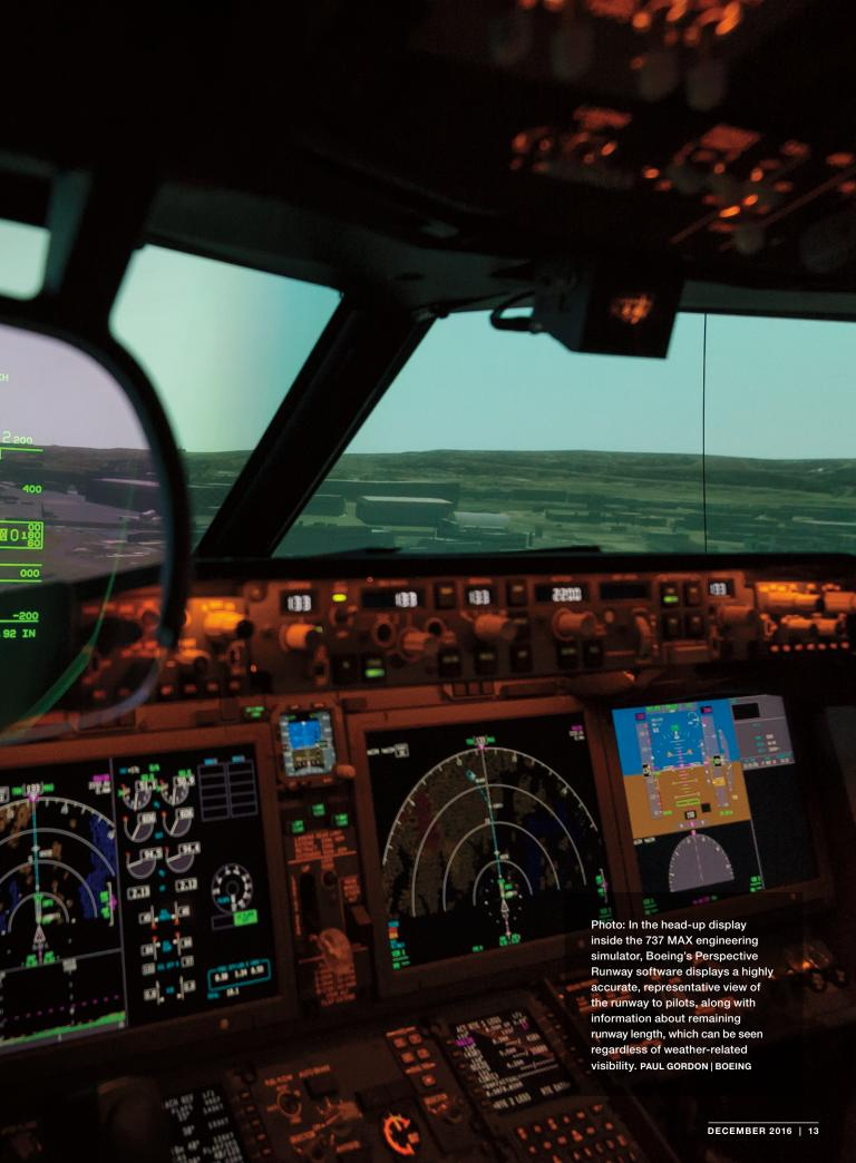
display, or HUD, on the flight deck to point pilots toward the runway even when the airplane is still miles from the airport. Information from a navigation database and airplane sensor data are used to project what Fleiger-Holmes calls a "virtual runway" on the HUD. It adds to information from the glideslope, which guides pilots to the correct altitude as they fly down the approach path.
